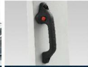
The armrest is equipped with horn switch for reversing, which makes driving safer;
