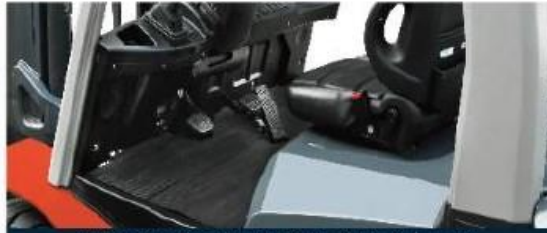
When the tilt cylinder sinks down in layout, the upper space of the bottom plate increases and the leg space is enlarged;
