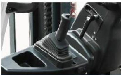
Ratchet type parking brake operating handle offers more labor-saving operation;
